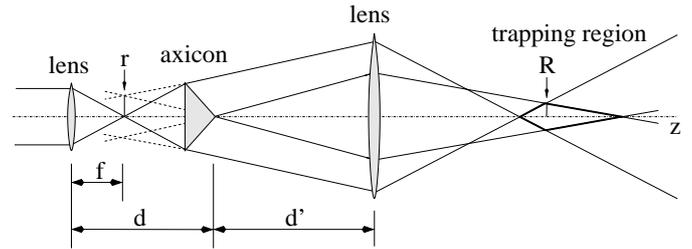
**Fig. 1.** Schematic of the experimental arrangement for the generation of a single-beam optical bottle intensity distribution. The first lens produces a “virtual” ring of radius  $r$ . The second lens images this ring and generates a dark region of radius  $R$ . In this figure  $f$  is the first lens focal length,  $d$  is the distance between the first lens and the axicon and  $d'$  is the distance between the axicon and the second lens.
